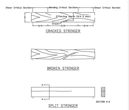
Figure 13.2-1. Cracked, Broken and Split Timber Stringer Defects
