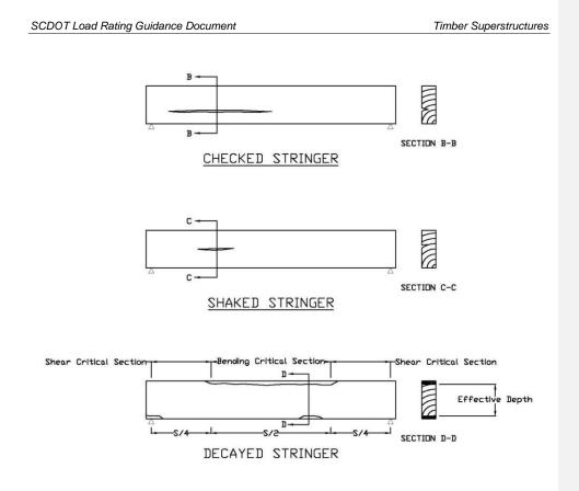
Figure 13.2-2. Checked, Shaked and Decayed Timber Stringer Defects
