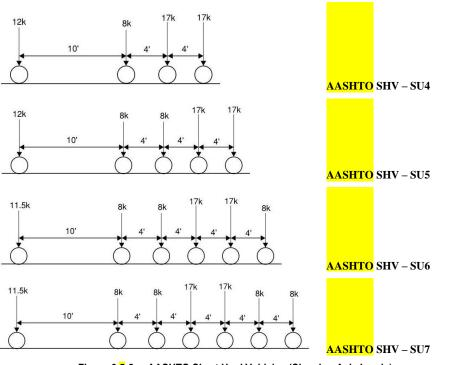
Figure 6.5-2a. AASHTO Short Haul Vehicles (Showing Axle Loads)
